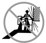
Be aware of crushing hazards when grasping the platform guard rail. During movement of the platform, occupants must keep all body parts inside the platform railing.
